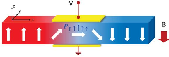
FIG. 1. Schematic of the one-dimensional multiferroic DW structure consisting of a Néel-type magnetic DW which induces an electric polarization (blue arrows) within the DW. A voltage is applied along the  $z$  direction, while the external magnetic field  $\mathbf{B}$  is kept in  $-\hat{z}$  direction. The white broad arrows denote the local spins in the wall.
