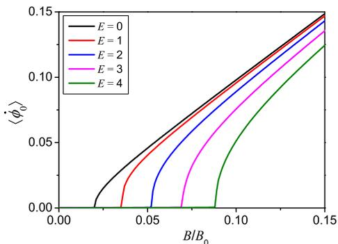
FIG. 2. The behavior of the time-averaged precession velocity  $\langle \dot{\phi}_0 \rangle$  as a function of magnetic field  $B$  at several applied electric field  $E$ .  $\langle \dot{\phi}_0 \rangle$  is given in units of  $K_{\perp} S / 2\hbar$ , the electric field  $E$  is given in units of  $E_0 = v_{\perp} / \gamma$ , and units  $B_0 = K_{\perp} S / 2g\hbar$ . The regime with  $\langle \dot{\phi}_0 \rangle = 0$  represents the stationary regime of the DW motion.
