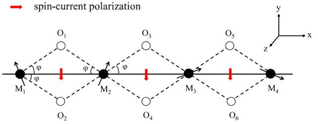
**Figure 7.** A schematic edge-shared MO<sub>2</sub> chain. The bridge oxygen atoms are symmetrically located beside the two sides of the magnetic metal atoms chain. In this case, the lattice-mediated contribution of the electric polarization is exactly cancelled. The nonvanish part of the polarization arise from the spin current, indicated by red arrows.
