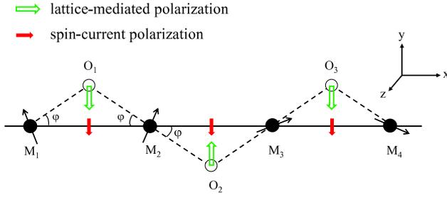
**Figure 6.** A sketch of the staggered M–O–M chain. The neighbor oxygen atoms of a given magnetic metal atom displace towards opposite directions. The spin-current polarization is uniform in each M–O–M cluster (red arrows), while lattice-mediated polarization is staggered (green arrows).
