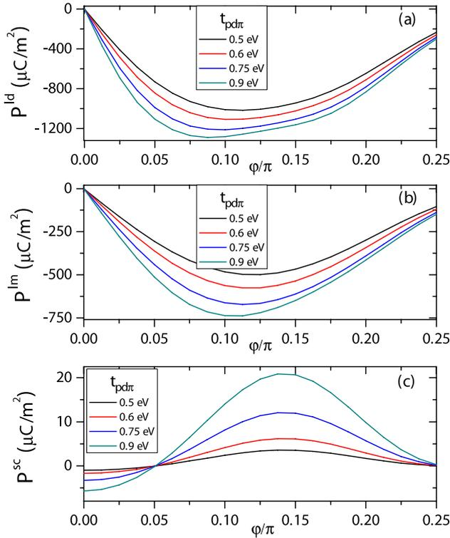
**Figure 8.** The  $\varphi$ -dependence of electric polarizations in uniform bending M–O–M chains (see figure 5). (a) Lattice-driven electric polarization. (b) Lattice-mediated polarization. (c) Spin-current polarization.
