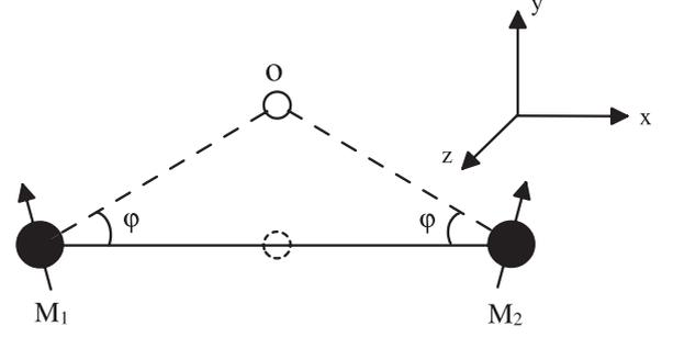
**Figure 3.** The three-atom M–O–M cluster model.  $M_1$  and  $M_2$  denote two transition metal ions with noncollinear magnetic moments. O represents a bridge oxygen atom which deviates from its centrosymmetric position (denoted by the dash circle) with a bond-bending angle  $\phi$ . The arrows on  $M_1$  and  $M_2$  indicate the spin direction. The three atoms of the cluster are assumed to be lying in the  $xy$  plane.
