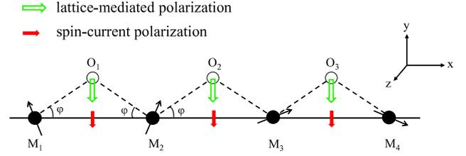
**Figure 5.** A sketch of the uniform bending M–O–M chain. All the bridge oxygen atoms deviate from the transition metal atoms chain in the same direction and lie within the  $xy$ -plane. And the spin spiral plane is the  $xy$ -plane. The spin-current and lattice-mediated polarization are denoted by red and green arrows, respectively.
