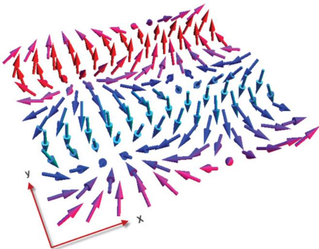
FIG. 2. (Color online) Schematic illustration of the spin order for the double periodic solution of the gauge Landau-Lifshitz equation.
