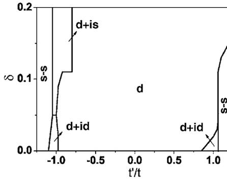
FIG. 2. Phase diagram of the  $t$ - $t'$ - $J$ - $J'$  model on a checkerboard lattice in parameter space of hole density  $\delta$  and  $t'/t$  obtained by the renormalized mean-field theory. The phases are indicated by their superconducting pairing symmetry defined in Table I and  $J'/J = (t'/t)^2$ .
