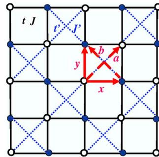
FIG. 1. (Color online) Schematic structure of 2D checkerboard lattice. Solid (open) circles represent sublattice A (B). The hopping integral and spin-spin coupling are  $t$  and  $J$  for the nearest neighbor links (solid lines) and  $t'$  and  $J'$  for the diagonal or next-nearest neighbor links (dashed lines), respectively.
