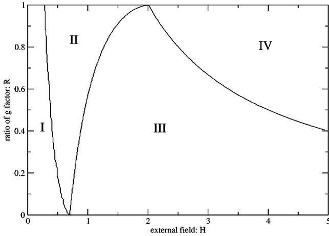
FIG. 2. Phase diagram of magnetic field  $H$  and the ratio of Landé  $g$  factors,  $R = g_t/g_s$ . There exist separated phases: (I) (SSP-WOP), (II) (SSP-OAP), (III) (SF-OP), and (IV) (SF-OF) in the region of  $0 < R < 1$ .
