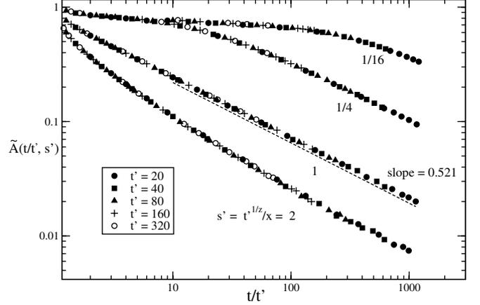
Fig. 3:  $\tilde{A}(t/t', s')$  is displayed for fixed values of  $s' = t'^{1/z}/x$  on a double-log scale. Data collapse is observed for different  $t'$ . The dashed line shows a power law fit.
